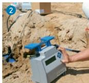
**MSA Plus control units.**Manual or automatic fusiondata input.
