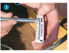
Automatic fusion data input. Easy and fast input of the necessary fusion data with the barcode reader.
