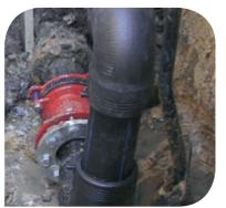
WAL/V leak clamps. WAL/V Single enables under pressure repair of leaking bell joint connections. WAL/V Double is the solution for leaking double socket connections. Both offering a range from DN80 - DN1200, for repair on all kinds of pipe materials.
