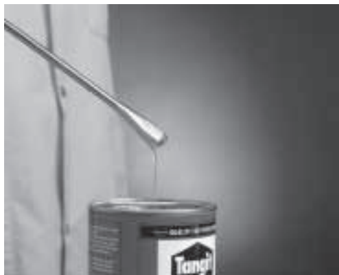
Checking the consistency of solvent cement
