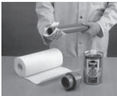
Cleaning the pipe and socket
